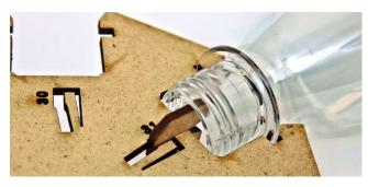
Figure 17: Laser-cut snap connectors are secured using a selflocking wedge.
