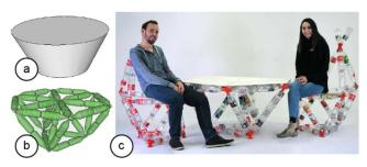
Figure 2: (a) TrussFab's converter automatically turns this 3D model of a coffee table, into (b) a sturdy tetrahedral honeycomb structure, (c) which fabricated serves as a functional table.
